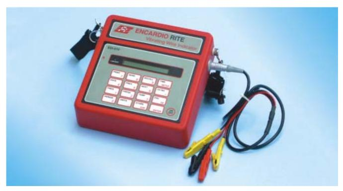
Model EDI-51V indicator can store calibration coefficients of maximum 500 number of sensors. It has capacity to store either 4500 readings from any one sensor or about 9 sets of readings from all 500 sensors. Each reading is stamped with date and time at which the measurement was taken.
