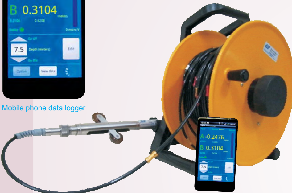
Easy to carry cable reel with provision to hold inclinometer probe
